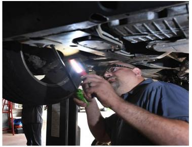
Rich Covelli, owner of Auto Medix, inspects a vehicle's front end suspension.
