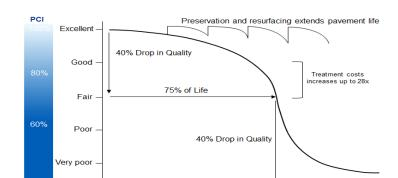
Chart 1. Pavement Condition Cycle Time with Treatment and Cost
