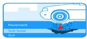
When temperatures rise, the thaw leaves cavities in the pavement. As traffic drives over the cavities, pavement is loosened and crushed, creating a pothole.
