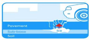
The water freezes and expands, making the cracks larger, and creating space for more moisture to collect. When the water freezes, it pushes pavement up and apart.
