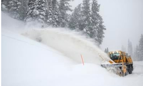
Richard Wilson drives WYDOT's rotary plow down the pass during a 2022 closure for avalanche control.
